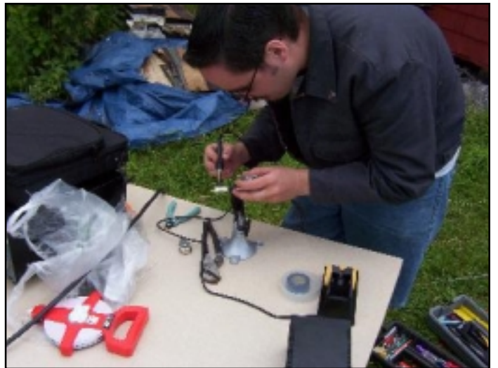
Greg, K2GTM, solders a PL259 onto a coax.
