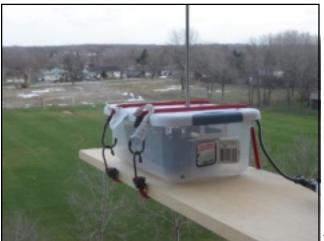
desirable to use the internal tuner as the Mark V RF power adjustment is not a smooth, linear operation with my external tuner. The Mark V operates at a maximum of 200 watts PEP SSB. The add on tuner limit is 150 watts PEP SSB. It is
