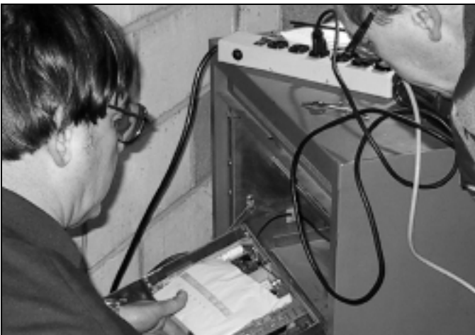
Dick, WB2DSS, installs the PL boards in the GE MastrII while Gil, W2EUP looks on.
